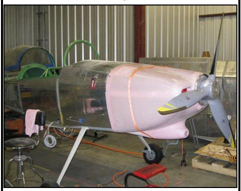
I now have the engine and prop for my RV8. The engine is an O-375 from AeroSport Power. The prop is from Catto Propellers, three-blade fixed pitch, composite with nickel leading edges. I recently received the mufflers for the exhaust.
